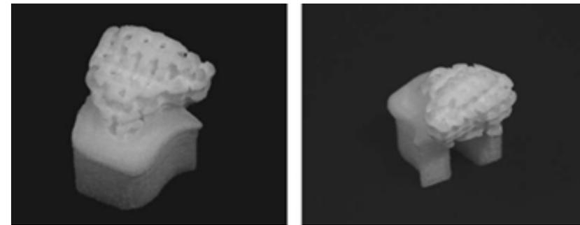
PCL printed by direct energy deposition technique [2]
