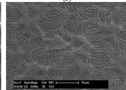
Surface profile of printed mesh samples
