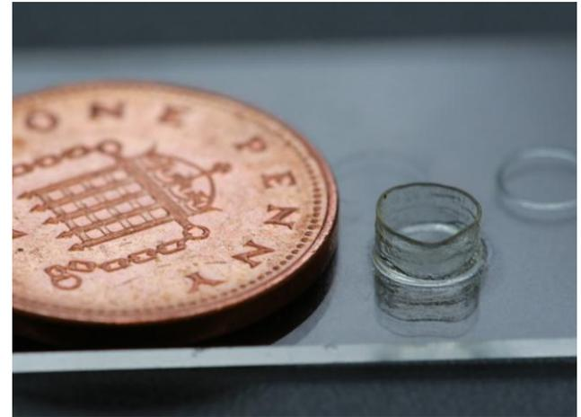
Image 1: Aprox. 120  $\mu\text{m}$  wall thickness cylinder printed with the rigid monomer
