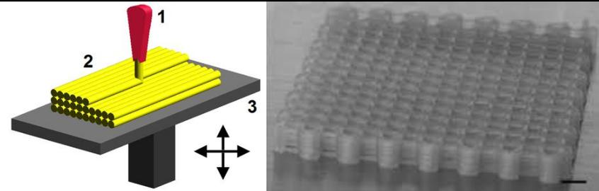
PCL printed by material extrusion technique [1]
